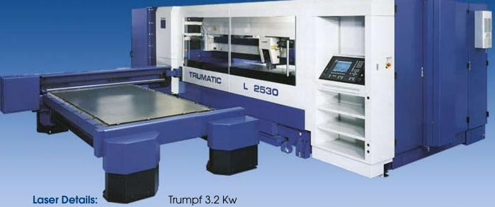
Bed Details: Cutting Thickness: Trumpf 3.2 Kw 2440mm x 1220mm sheet size 20mm Mild Steel / 12mm Stainless Steel / 8mm Aluminium
